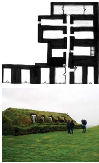
GLAUMBAR AT SKAGAFJÖRDUR A large farmstead of 14 houses, in excellent repair and walls built almost exclusively of turf.
