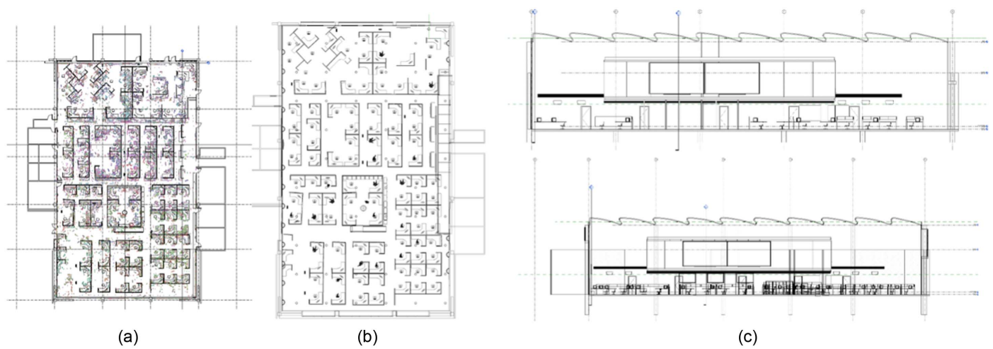
Fig. 7. Model-authoring software system integrates with point cloud data: (a) modeling based on point cloud; (b) detailed BIM model; and (c) section views.
